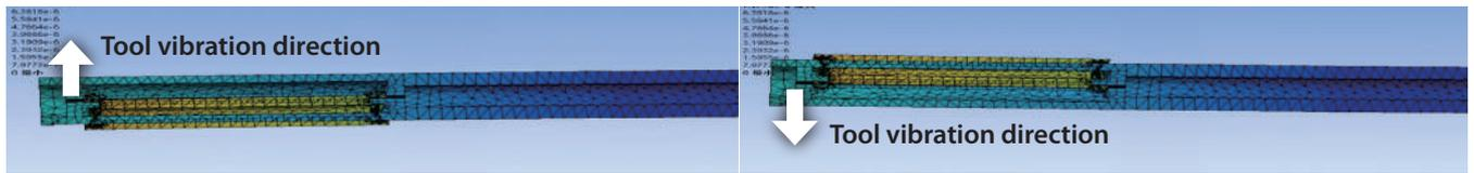
The damper vibrates late against the shank. Effective for vibration damping
