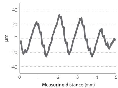
Cutting Conditions:  $V_c = 150$  m/min,  $a_p = 0.4$  mm,  $f = 0.15$  mm/rev Workpiece: SCM435 Overhang length 320 mm
