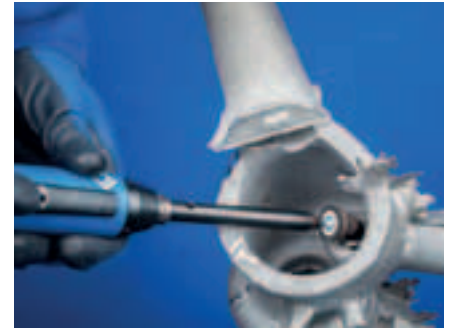
Extension SPV 150-3 S6 for shank diameter 3 mm
