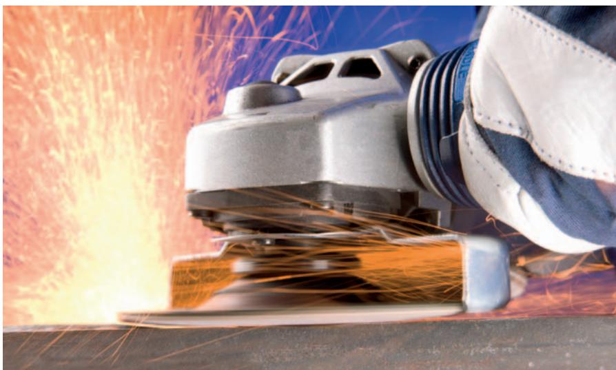
The innovative cooling and mounting systems allow grinding at very flat angles and the optimum utilization of the abrasives available.
