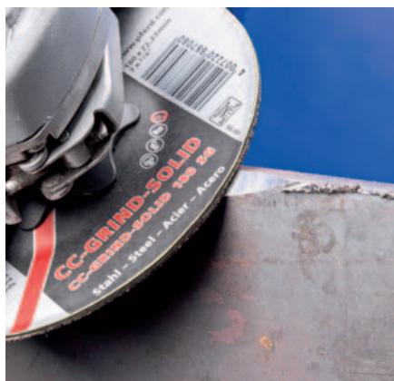
The CC-GRIND system was **specially developed for aggressive and economic grinding** with ultimate stock removal rates and very good tool life in surface and edge grinding applications. The special version of the respective grinding disc combined with the matching mounting system guarantees maximum stock removal performance in a very short time.
