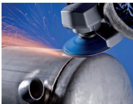
PFERD INOX version for cool grinding with very good stock removal on stainless steel (INOX).
