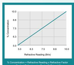
Coolant Refractometer Factor % Brix = 1.0
