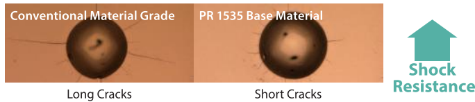
Cracking Comparison by Diamond Indenter (Internal evaluation)
